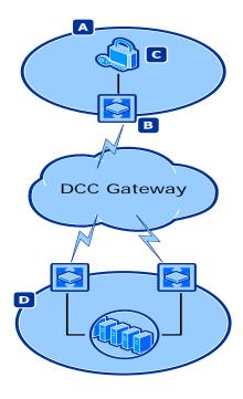
In this example, a single connection to the DCC Gateway is made from the DCC Gateway Party location [A] to DCC MPLS network and onwards to the DCC data centres [D].
