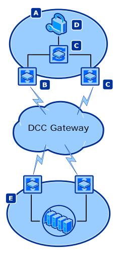
In this example the DCC Gateway Party data centre [A] is linked using diversely routed links and dual routers [B,C] to the DCC MPLS network and onwards to the DCC data centres
