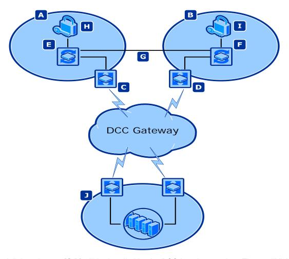
A link and router [C.D] will be installed by the DCC into the two sites. These will link to a DCC Gateway Party provided layer-2 switch at each site [E,F] and connect to the Party PEP [H,I].
